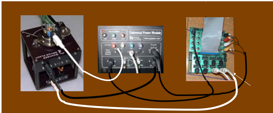
Figure 1.10 Wiring diagram for Flexible Link Project.
