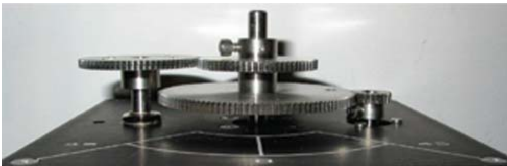
Figure 9 High gear ratio configuration
