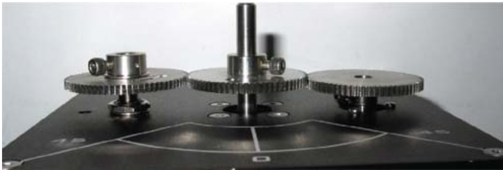
Figure 8 Low gear ratio configuration
