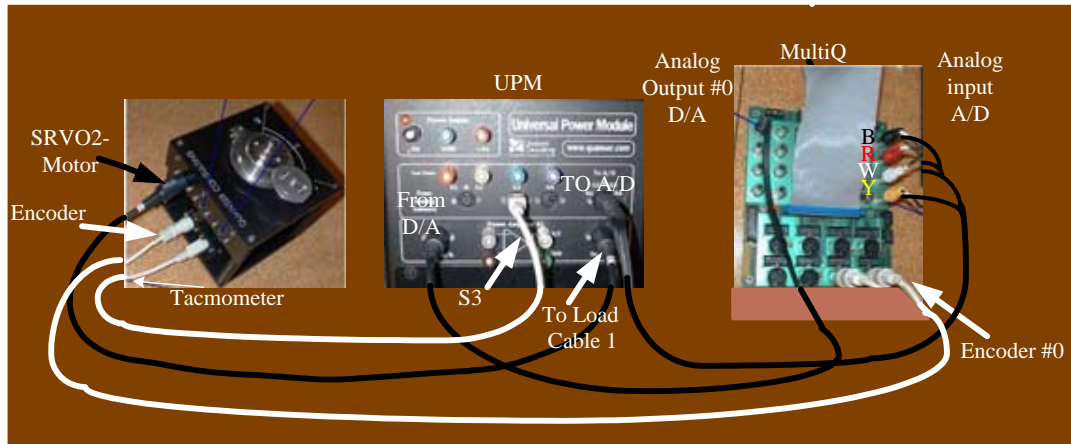
Figure 6.8 Wiring diagram for servo motor speed control system.
