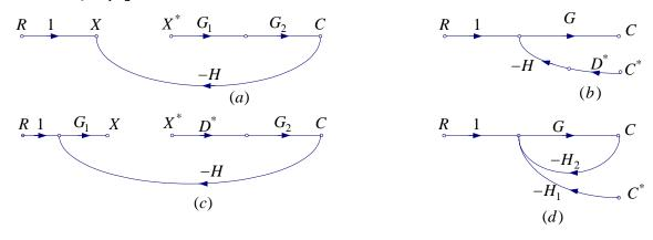
Determine  $\frac{C(z)}{R(z)}$  for each block diagram.
